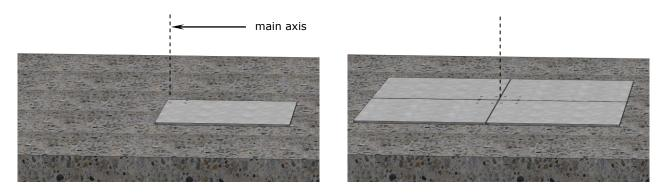
2. Determine the correct position of SZ272/SZ274 after careful calculation of the main axis of the parasol. Allow enough clearance between parasols or from walls.
