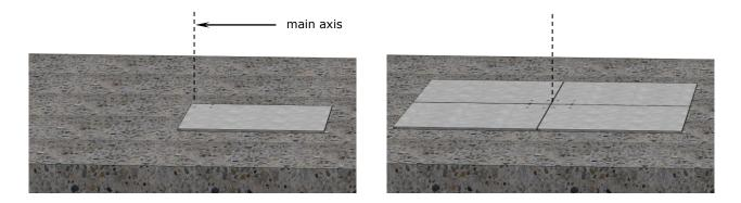
2. Determine the correct position of SZ273/SZ275 after careful calculation of the main axis of the parasol. Allow enough clearance between parasols or from walls.
