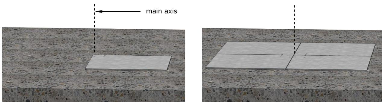
2. Determine the correct position of SZ272/SZ274 after careful calculation of the main axis of the parasol. Allow enough clearance between parasols or from walls.
