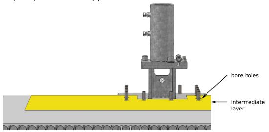
6. Use the loos flanges to fix the intermediate layer. Make sure to position the loose flanges with the flanging radius facing outwards and the corner bevels pointing down.
