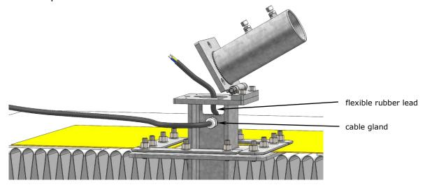
2. The connection of the flexible rubber lead and power supply for the parasol must be absolutely waterproof. The ground cable (for heavy current: min. 5-pole, min. 4mm², cable cross section) must be laid to suit the electric load and the length of the lead wire by a qualified electrician.
