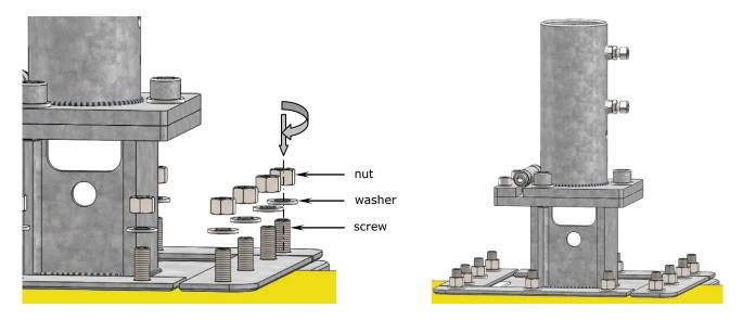
8. Due to the manufacturing process, the screws are not galvanised and thus are not protected from corrosion. Therefore all 12 screws must now be coated with liquid zinc. This is required to make sure the threads will not rust and remain functional.
