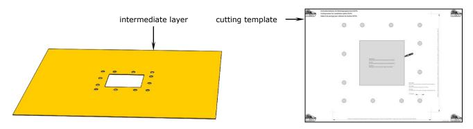
5. Put the intermediate layer over the upper tube and place the screws into the bore holes. Depending on the waterproofing material there is an additional layer or a reinforcement required, see DIN 18195, part 9.
