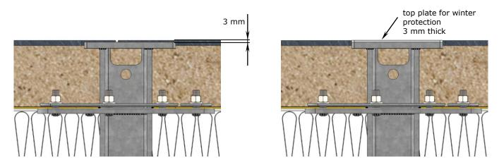
2. Lay the stone slabs and saw away the corners of those that are to fit round the SZ194. Make sure that the SZ194 sits flush.
