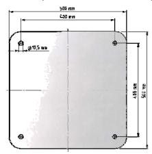
2. Screw the anchor plate onto the foundation. If you use anchor bolts provided by other manufacturers, please observe their instructions. Anchor bolts supplied by MAY should be mounted as follows:
