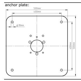
When drilling the heavy-duty anchor bolts into the designated site position, use the anchor plate as a drilling jig. You will need 4 heavy-duty anchor bolts. Available in stainless steel A4, art. no. 200900.
