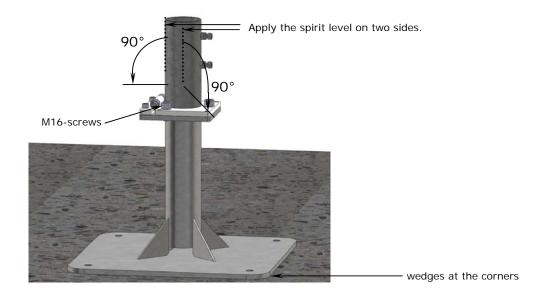
4. When setting the SZ127 / SZ027, make sure that the ground-level plate of the bottom component is (almost) flush (-3 mm) with the terrace floor surface.
