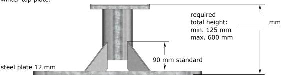
In case the "height of the lower part" needs to be lower than 125 mm, option SZ027 must be used.
