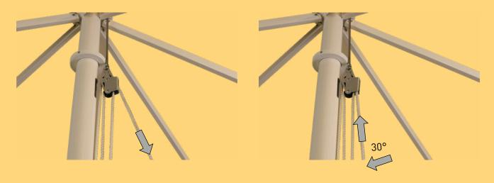
FILIUS Pagoda with crank drive FK: Insert the crank or the drill bit into the designated bore of the canopy mechanism and close the parasol by turning it anti-clockwise.
