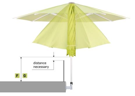
Consider the offset of the DMZ125. If the anchor plate is mounted flush with the top edge the measures F and G decrease about 26 cm. In case the parasol roof collides with the balustrade, a centre pole extension may help. Using a DMZ170 instead of the DMZ125 may also be an option.
