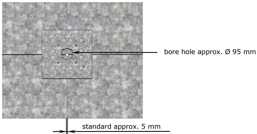
2. If a bigger centre bore hole or a larger distance between the steel plates is required, a flange plate with long holes can be ordered optionally (art. no. 357570). This allows to move a single base plate or all 4 base plates, which is not related with any restrictions in mechanical capacity. All instructions of this manual remain applicable.
