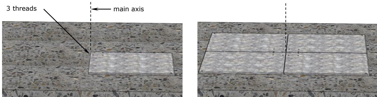
2. Determine the correct position of AZ246 / AZ247 / AZ248 / AZ249 after careful calculation of the main axis of the parasol. Allow enough clearance between parasols or from walls.
