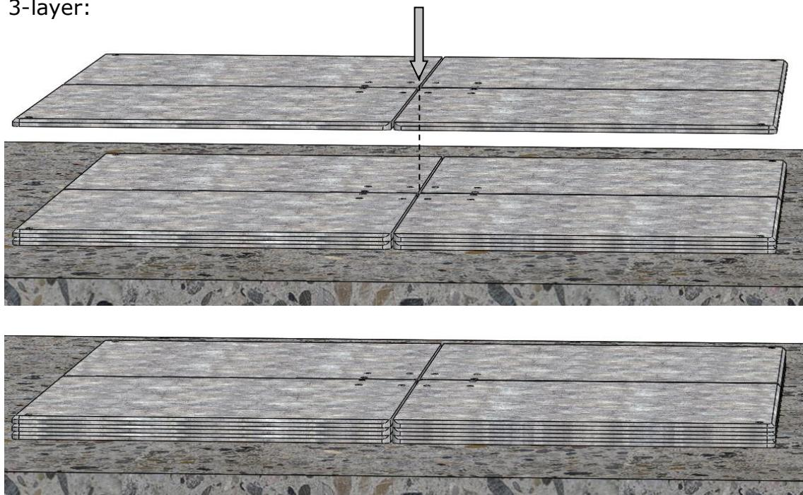
5. Place the top layer of steel plates with the countersinking at the edges facing up.
