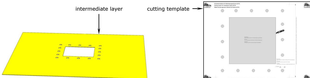
5. Put the intermediate layer over the upper tube and place the screws into the bore holes. Depending on the waterproofing material there is an additional layer or a reinforcement required, see DIN 18195, part 9.
