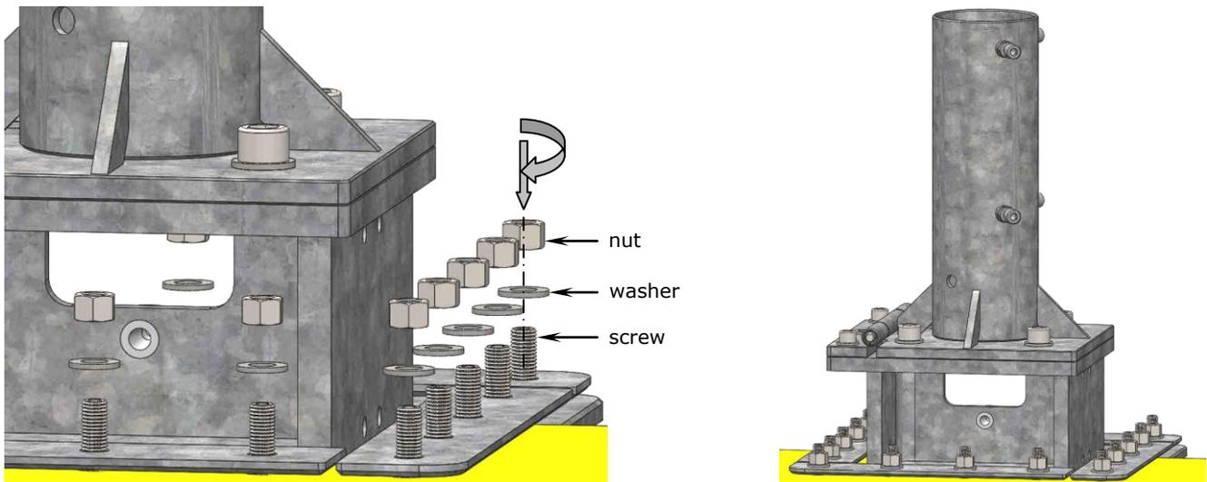
8. Due to the manufacturing process, the screws are not galvanised and thus are not protected from corrosion. Therefore all 12 screws must now be coated with liquid zinc. This is required to make sure the threads will not rust and remain functional.
