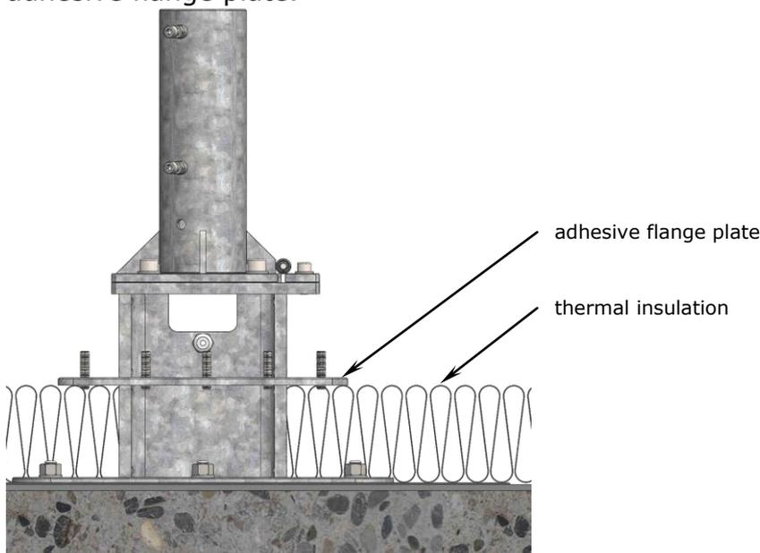
3. Spread out the waterproofing sealing membrane on the insulation layer. When doing so, cut out a hole in the membrane so that it will fit exactly round the adhesive flange and thus a butt joint. Depending on the waterproofing membrane used, it may be necessary to reinforce with further layers.
