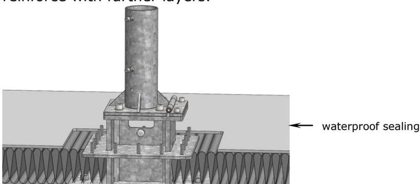
4. Prepare the intermediate layer. Cut out a 1x1m piece of the waterproofing material. Use the provided cutting template (DIN-A3) to prepare the squared cut out and the 12 bore holes. Tools: knife and punch Ø14 mm.
