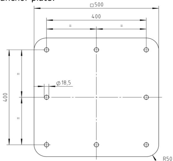
When drilling the heavy-duty anchor bolts into the designated site position, use the anchor plate as a drilling jig. You will need 8 heavy-duty anchor bolts. Available in stainless steel A4, art. no. 200900, 2 packages.
