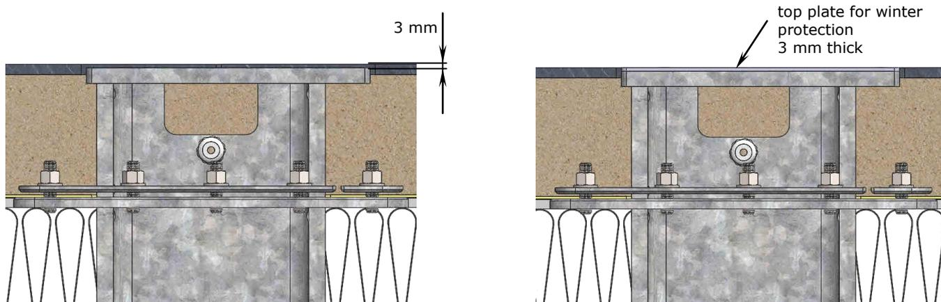
2. Lay the stone slabs and saw away the corners of those that are to fit round the AZ194. Make sure that the AZ194 sits flush.
