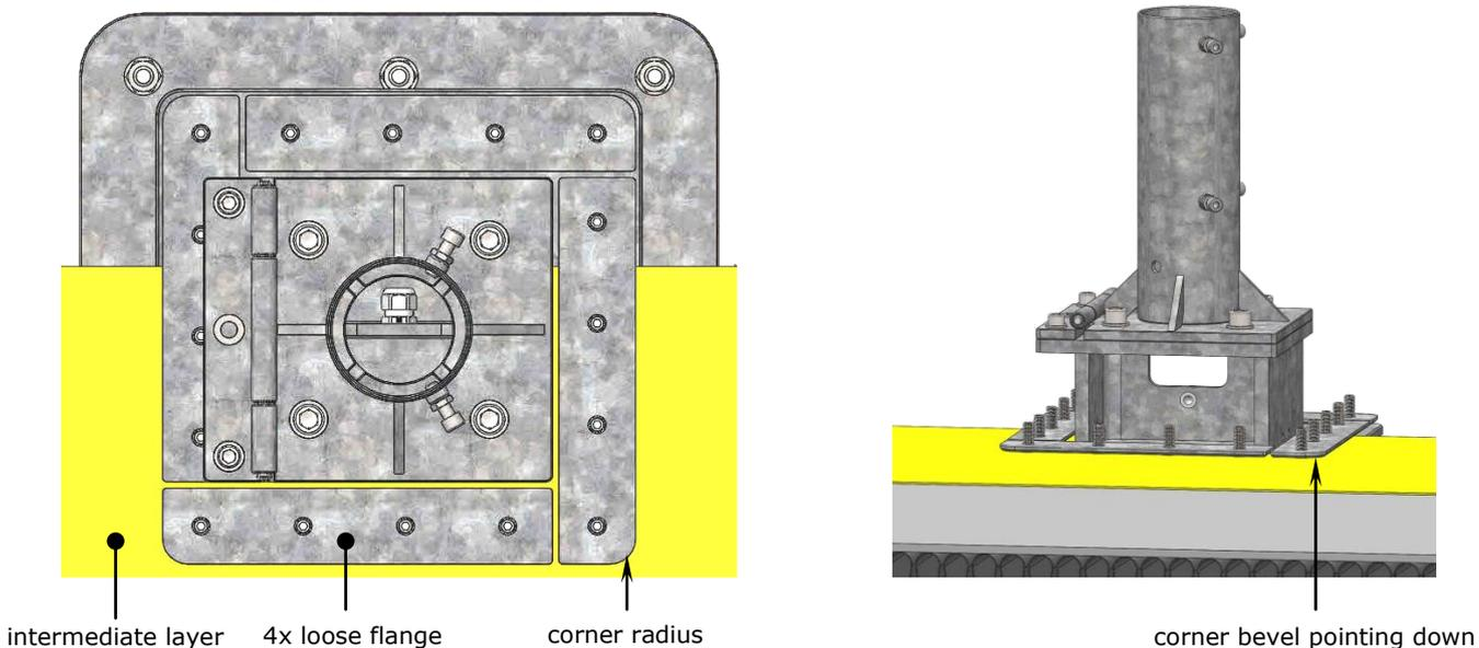
7. Tighten the four loose flanges. Put a washer on each of the 16 screws and screw on the nuts accordingly. The nut torque depends on the selected waterproofing material, according to DIN 18195, part 9, table 2.
