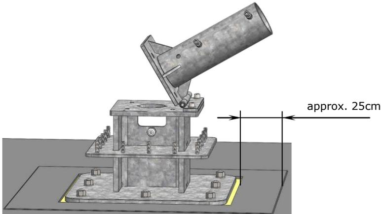
2. Fill up the thermal insulation course with insulating material as far as the bottom of the adhesive flange plate.
