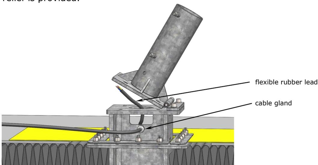
2. The connection of the flexible rubber lead and power supply for the parasol must be absolutely waterproof. The ground cable (for heavy current: min. 5-pole, min. 4mm<sup>2</sup>, cable cross section) must be laid to suit the electric load and the length of the lead wire by a qualified electrician.
