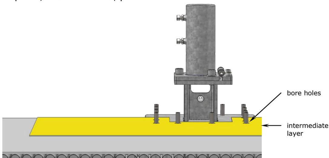
6. Use the loose flanges to fix the intermediate layer. Make sure to position the loose flanges with the flanging radius facing outwards and the corner bevels pointing down.
