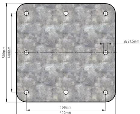
2. Screw the anchor plate onto the reinforced concrete surface. If you use anchor bolts provided by other manufacturers, please observe their instructions. Anchor bolts supplied by MAY should be mounted as follows:
