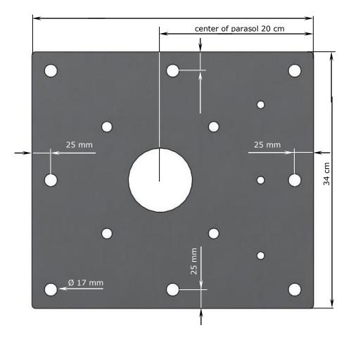
5. Screw the anchor plate onto the foundation. If you use anchor bolts provided by other manufacturers, please observe their instructions. Anchor bolts supplied by MAY should be mounted as follows:
