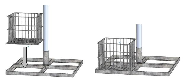
3. Get the stones you would like to use. The grain size must not be less than 60/90mm or at least larger than the wire mesh size 50 mm. In case of a grain size of 60/90 mm the filling reaches a load of approximately 110 kg. If required, please follow the table below:
